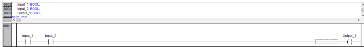
Figure 2.3: AND – logic operation.
