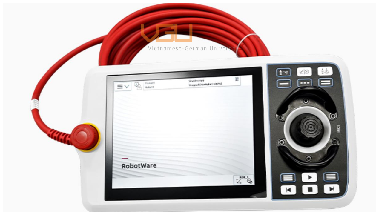
Figure 2.14: ABB's Omnicore FlexPendant
