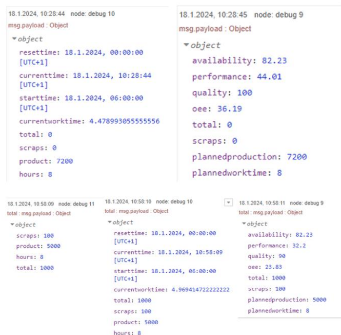
Figure 25: Result when pressing "Refresh" button (above) and result when receiving input from Phase 1 (below)
