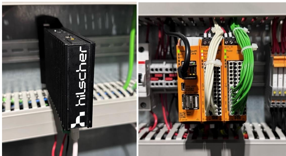
Figure 7: netFIELD Compact X8M (left) and RevPi Core (right) in LFF
