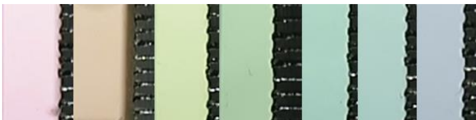
Figure 16: Recorded color profile of buffer solution mixed with universal indicator from pH 4, 5, 6, 7, 8, 9, 10 (left to right)
