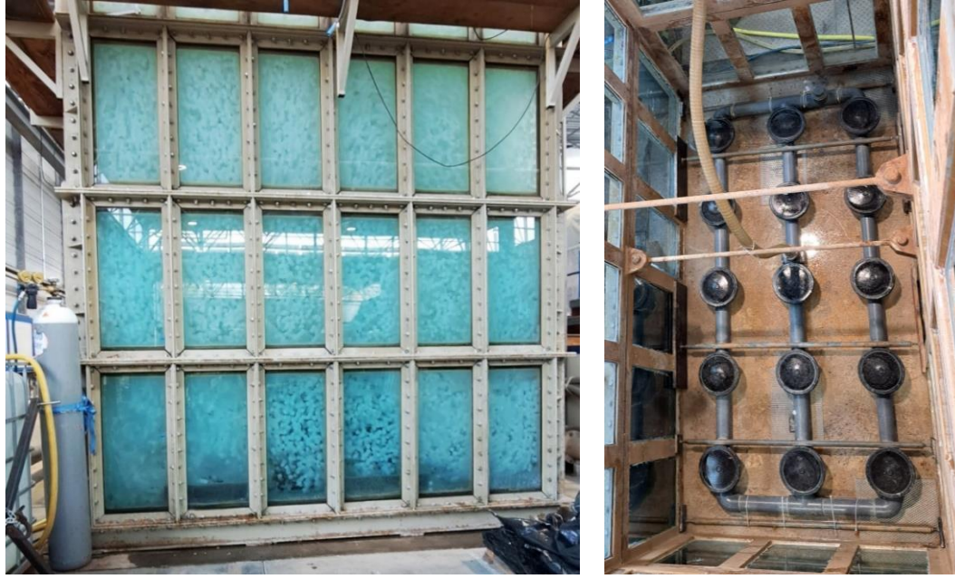
Figure 16. Experimental setup of the pilot-scale MBBR
