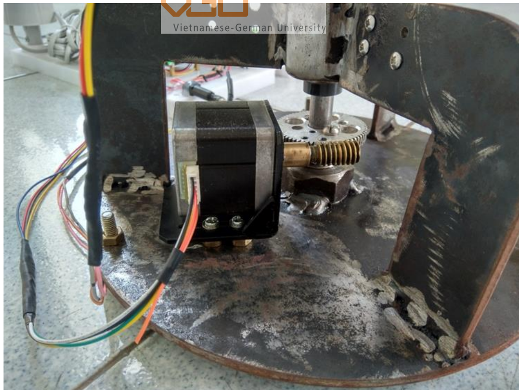
Figure 4.2: Stepper motor and worm gear system
