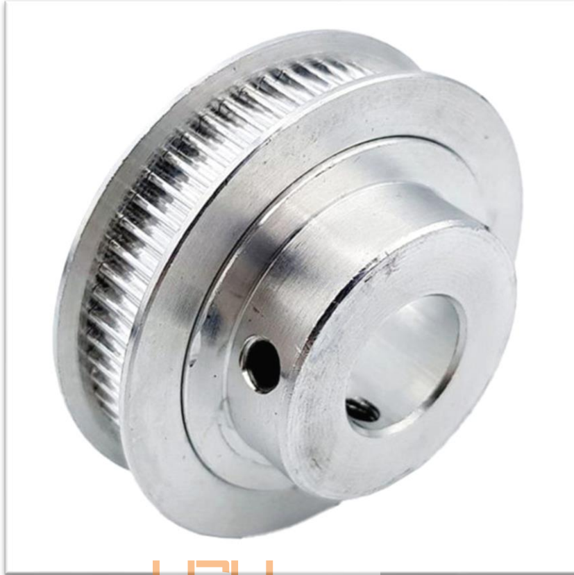
Figure 5.3: Part 40-GT2 60Teeth Bore 12mm Timing Pulley Wheel
