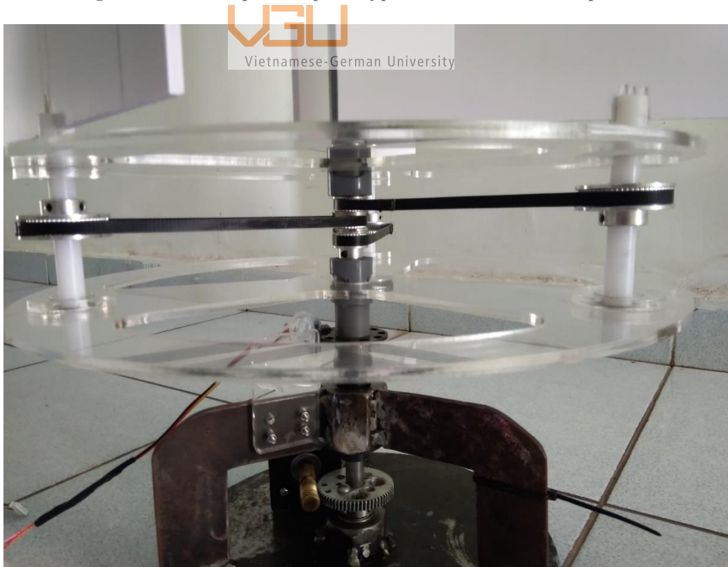
Figure 5.9: GT2 Timing Pulley system
