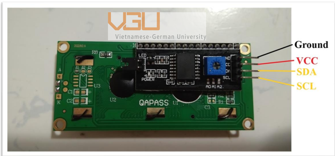
Figure 3.12: I2C connected to LCD with 4 pins output
