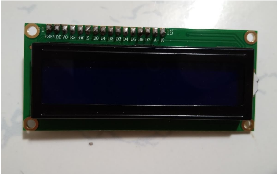
Figure 3.11: LCD screen with 16 pins
