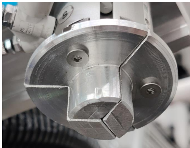
Figure 68: Flat finger to ensure the fitness of the Cage
