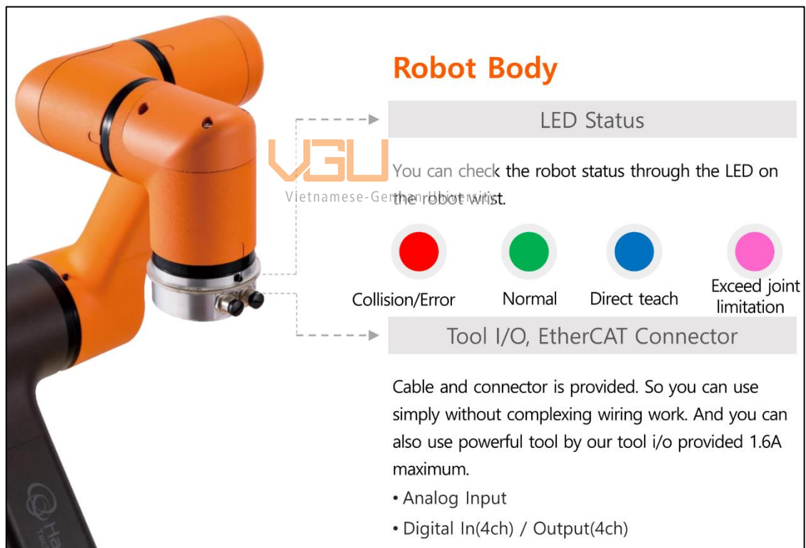
Figure 17: Signal status with Input- Output control of HCR-5 Cobot
