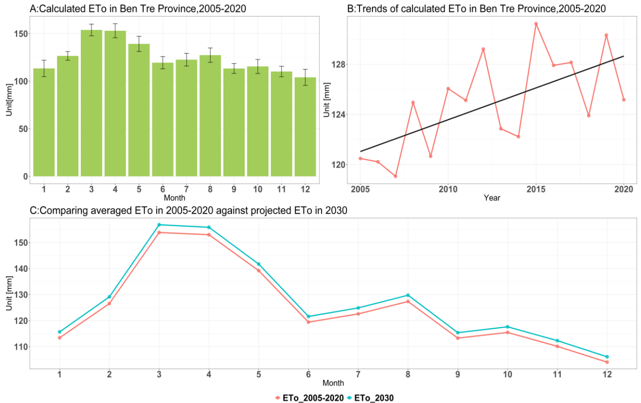
Fig. 15. (A) Variations of monthly average ET_0 from 2005 to 2020, (B) annual ET_0 trends from 2005 to 2020, and (C) comparing the historical monthly averaged ET_0 and projected ET_0 by 2030.
