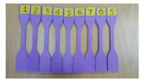
Fig. 2 Fabricated sample of PLA materials
