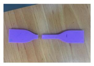
Fig. 3 Specimens after tensile test
