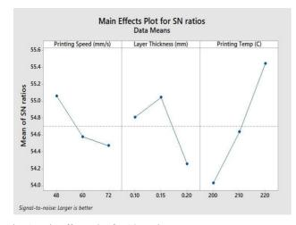
Fig. 4 Main effects plot for S/N ratios
