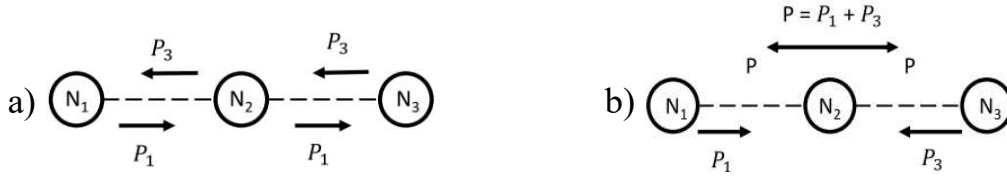
Figure 1: Simple data transmission model for three nodes. a) Without COPE; b) With COPE.
