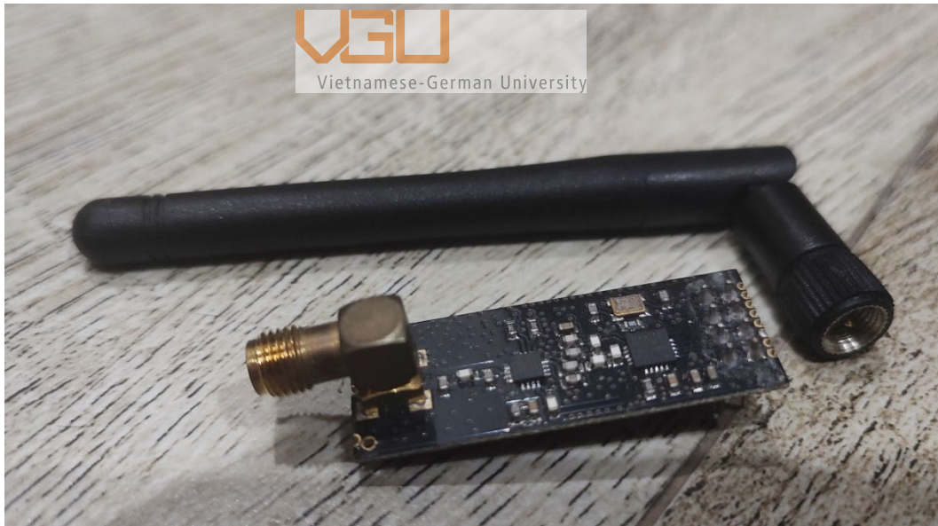
Figure 4.1: nRF24L01 module + PA + LNA + detachable antenna (Photo taken by the author at Vietnamese German University)
