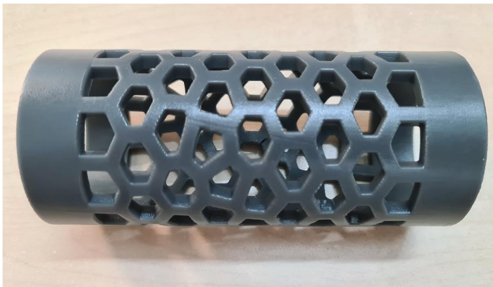
Figure 4.3 SLA printed test tube
