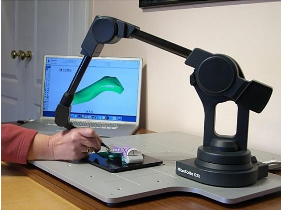
Figure 2.4 Contact-based scanning [Source: 3D-Prototype]
