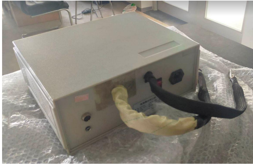
Figure 33: The behind of generator for battery spot welding machine
