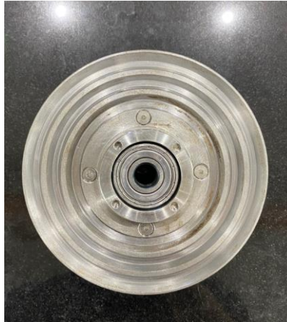
Figure 6.2: Assembly of tooth-shaped disc and MRB shaft
