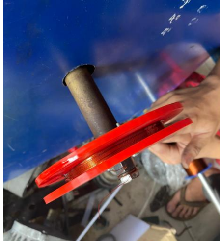
Figure 6.5: Wrapping copper wire on the coil mold
