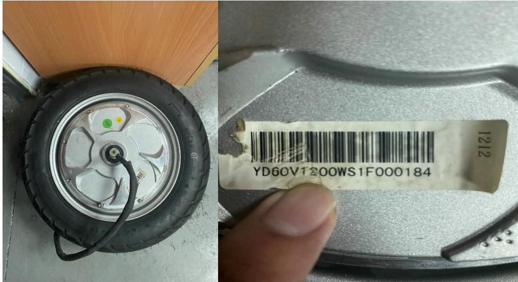
Figure 3.2: Back wheel and motor's parameter
