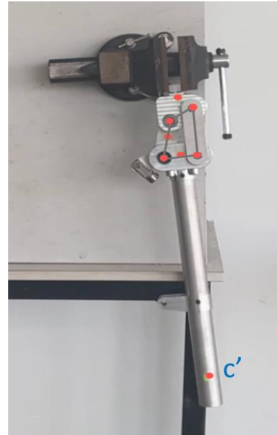
Figure 100 Prosthetic knee at the end of swing
