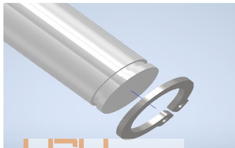
Figure 94 Shaft locked by an M8 retainer Vietnamese-German University
