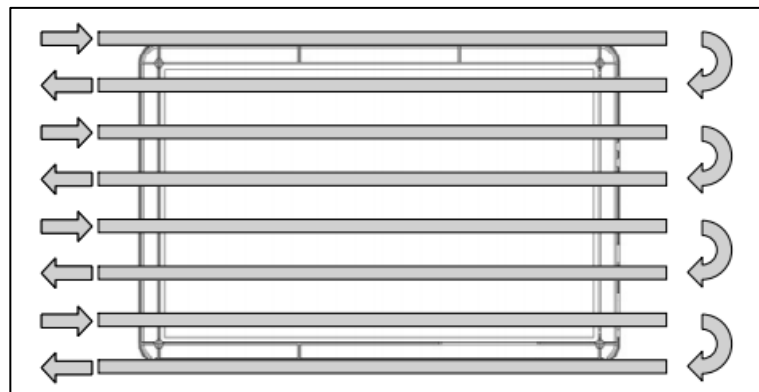
Figure 4-7: The cooling system with short return loop
