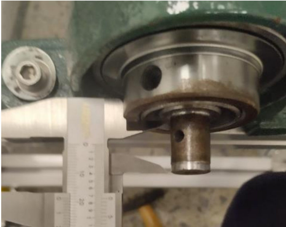
Figure 5. 8 Connecting section of drive shaft
