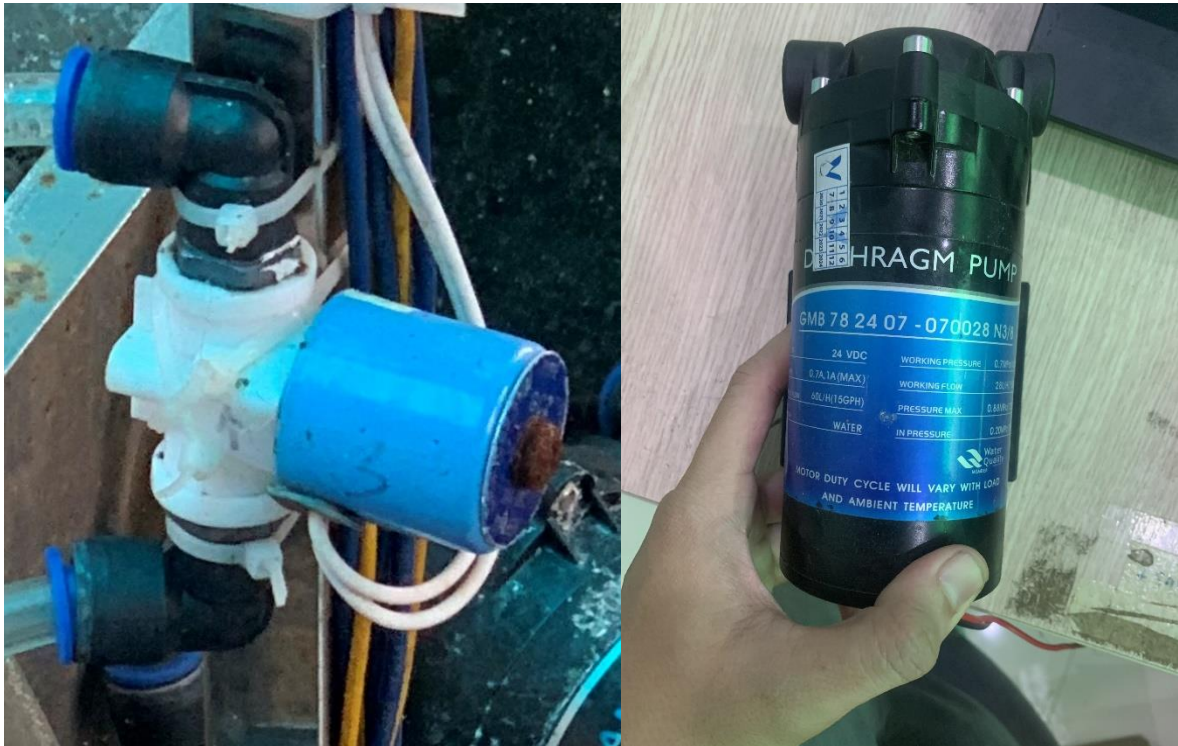
Figure 26: solenoid valve and diaphragm pump
