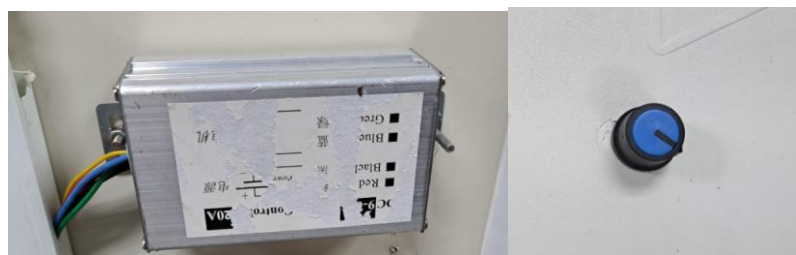
Figure 6-8 Actuator control module and control knob
