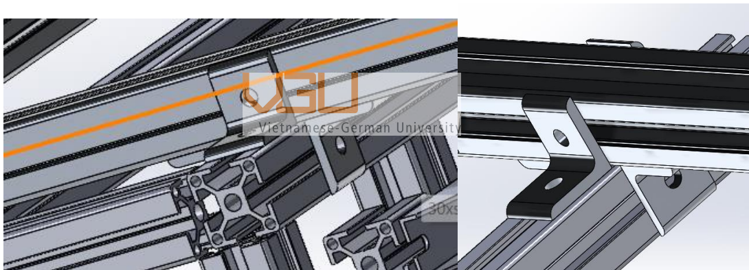
Figure 5-42 Width adjustable using bracket
