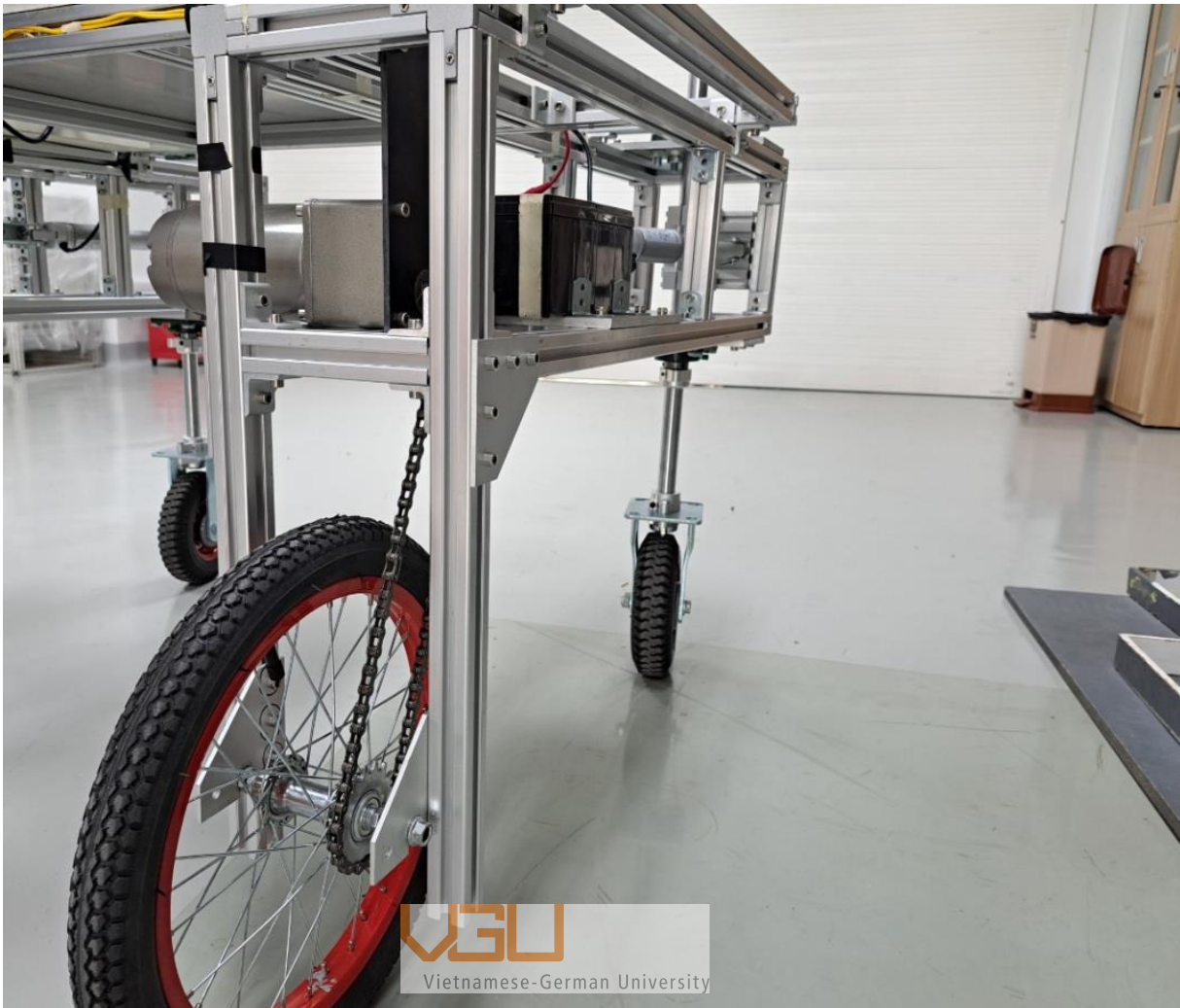
Figure 5-41 The motor frame and the steering frame after installation
