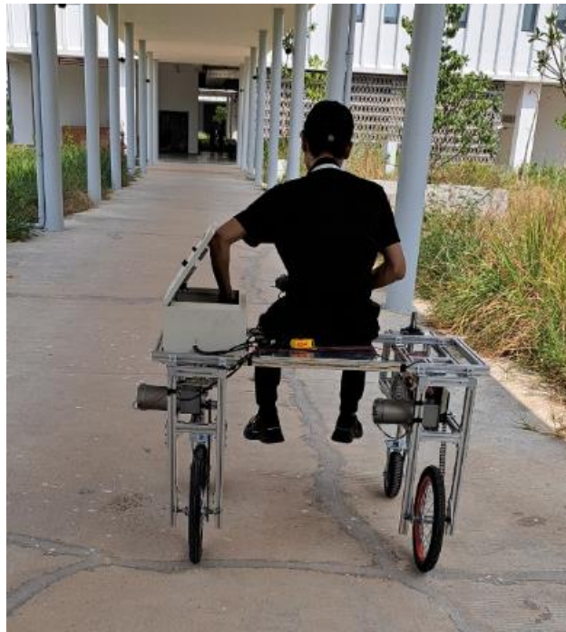
Figure 7-2 Testing loading capacities
