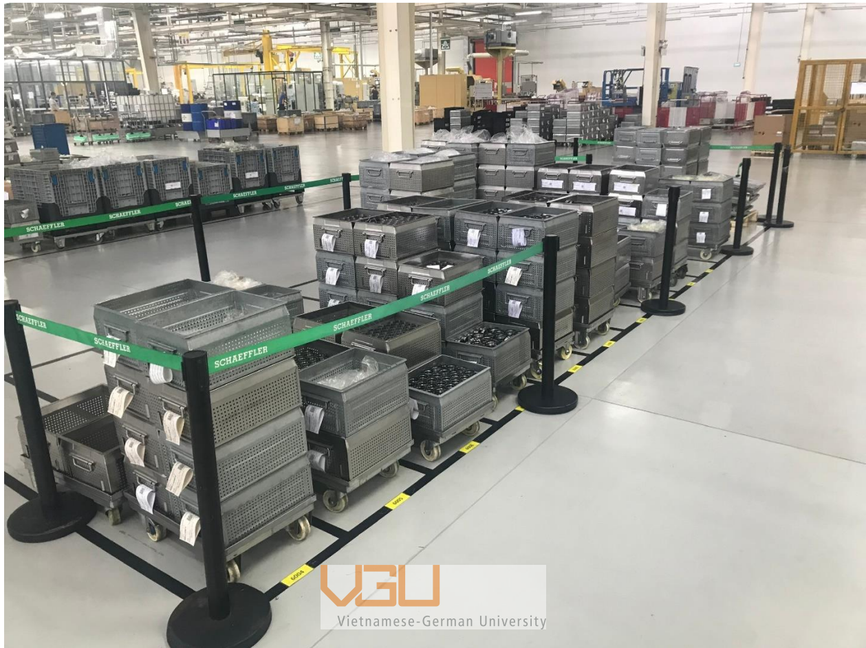
Figure 21. New layout for WIP area before assembly process
