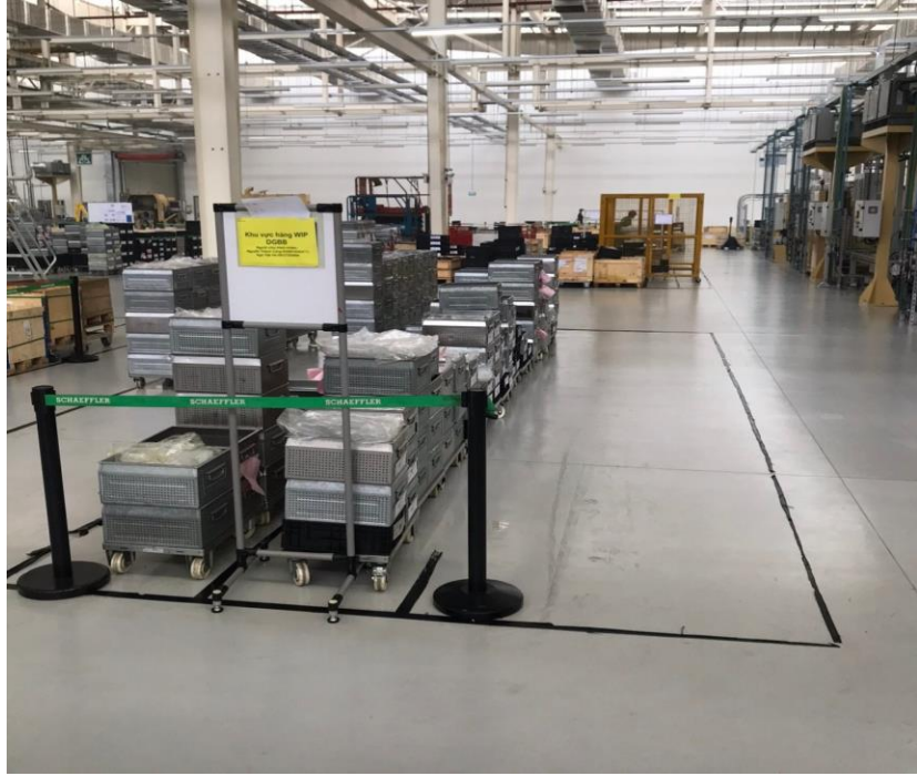
Figure 17. WIP area before assembly process without proper layout
