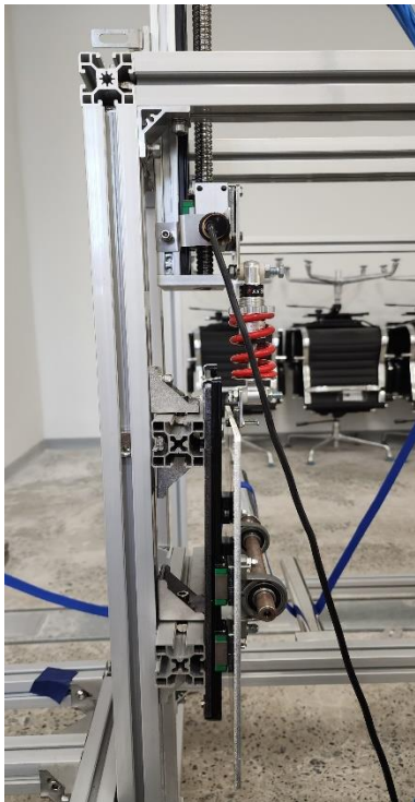
Figure 102 Dancer roller is at home position
