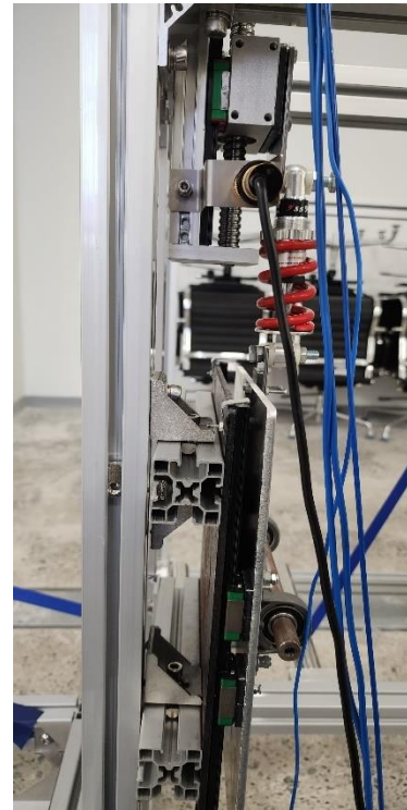
Figure 101 Dancer roller is at the highest point
