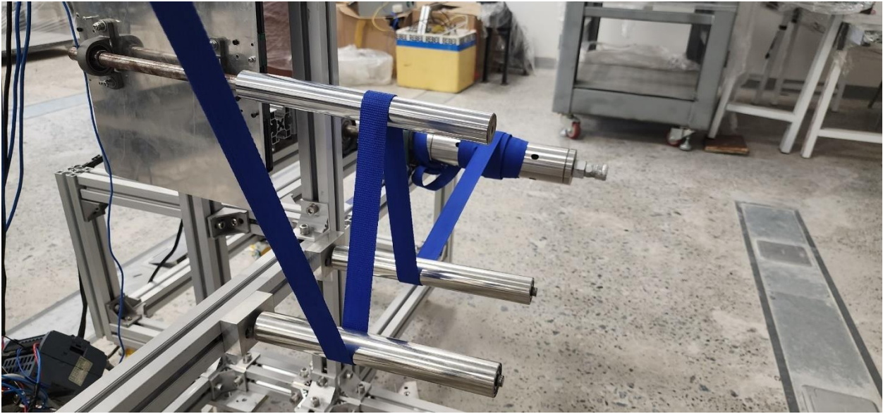
Figure 103 Load the tension to the dancer roller
