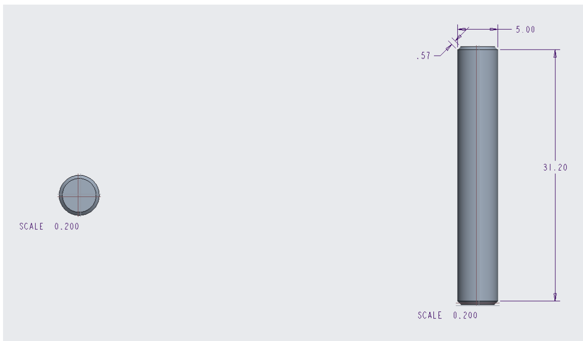
Figure 12. Design of the steel pin
