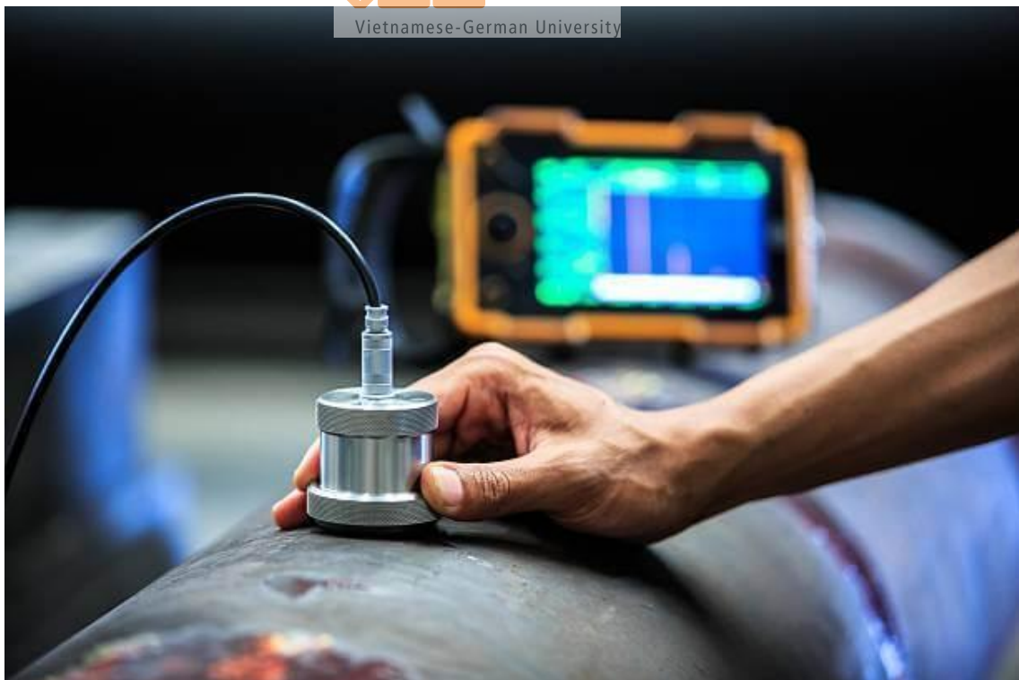
Figure 2: Applying ultrasonic testing on material surface [8]
