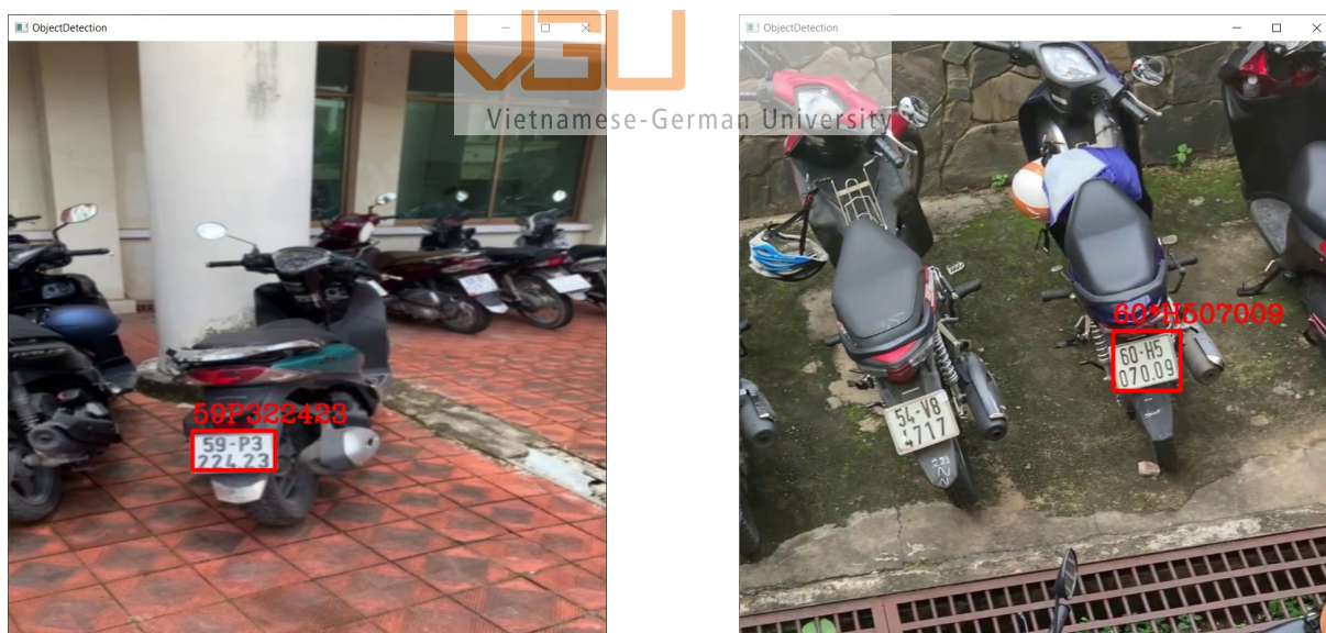
Figure 40: License Plate Recognition using EasyOCR
