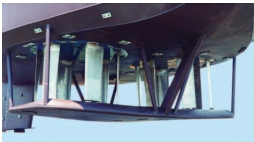
Figure 24: Voith-Schneider propulsion system [35].
