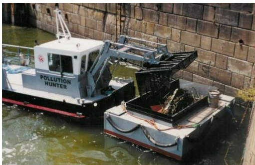
Figure 19: On the left, a weed tow boat, named “Pollution Hunter” by Water Witch, is unloading the bucket. On the right is a photo of using truck to unload a full barge.
