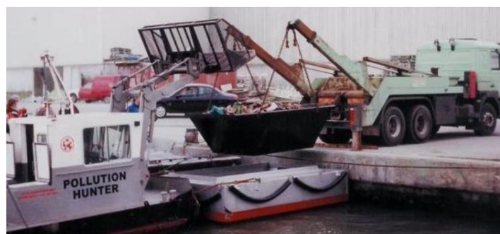
Figure 19: On the left, a weed tow boat, named “Pollution Hunter” by Water Witch, is unloading the bucket. On the right is a photo of using truck to unload a full barge.
