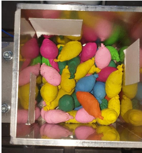
Figure 4-6: Small balloons being packed into the stator arm
