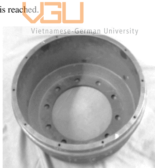
Figure 2-6: Brake drum with cavities on the wall for application of particle damping (Xia, et al., 2011)
