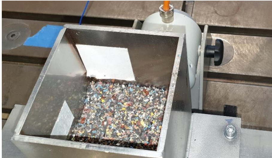
Figure 4-2: Filling the stator arm with 400 mL rubber
