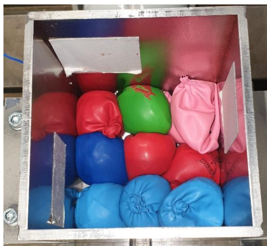
Figure 4-5: Big balloons being packed into the stator arm
