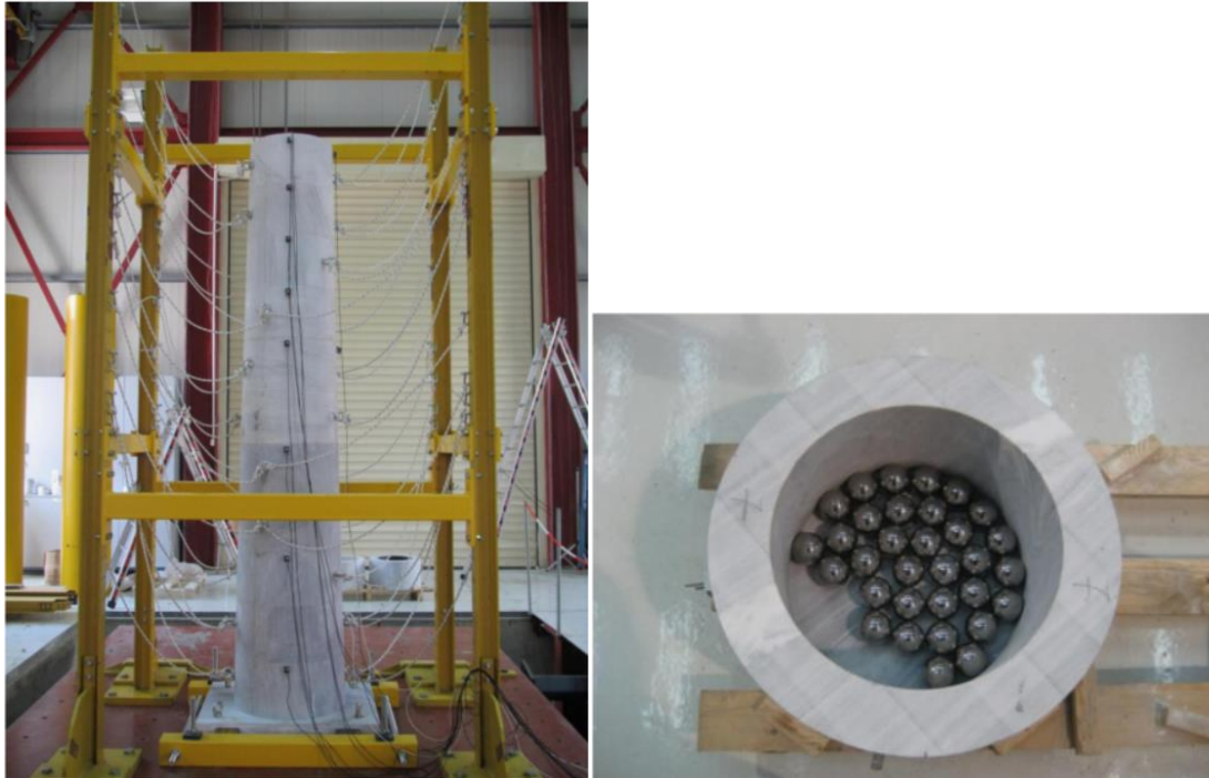
Figure 2-13: Experimental set up to study the seismic protection of PD (Papalou, et al., 2015)
