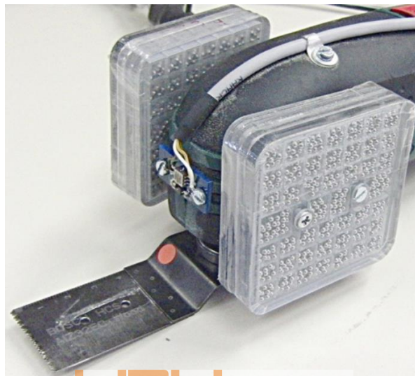
Figure 2-7: An oscillatory saw with prototype particle dampers attached (Heckel, et al., 2012)
