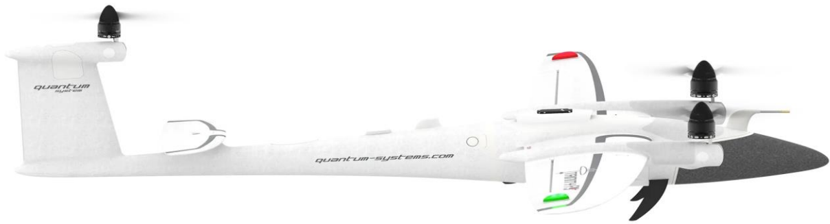
Figure 9: Trinity F90Plus mapping drone [Retrieved from (Quantum-Systems, 2022)]
