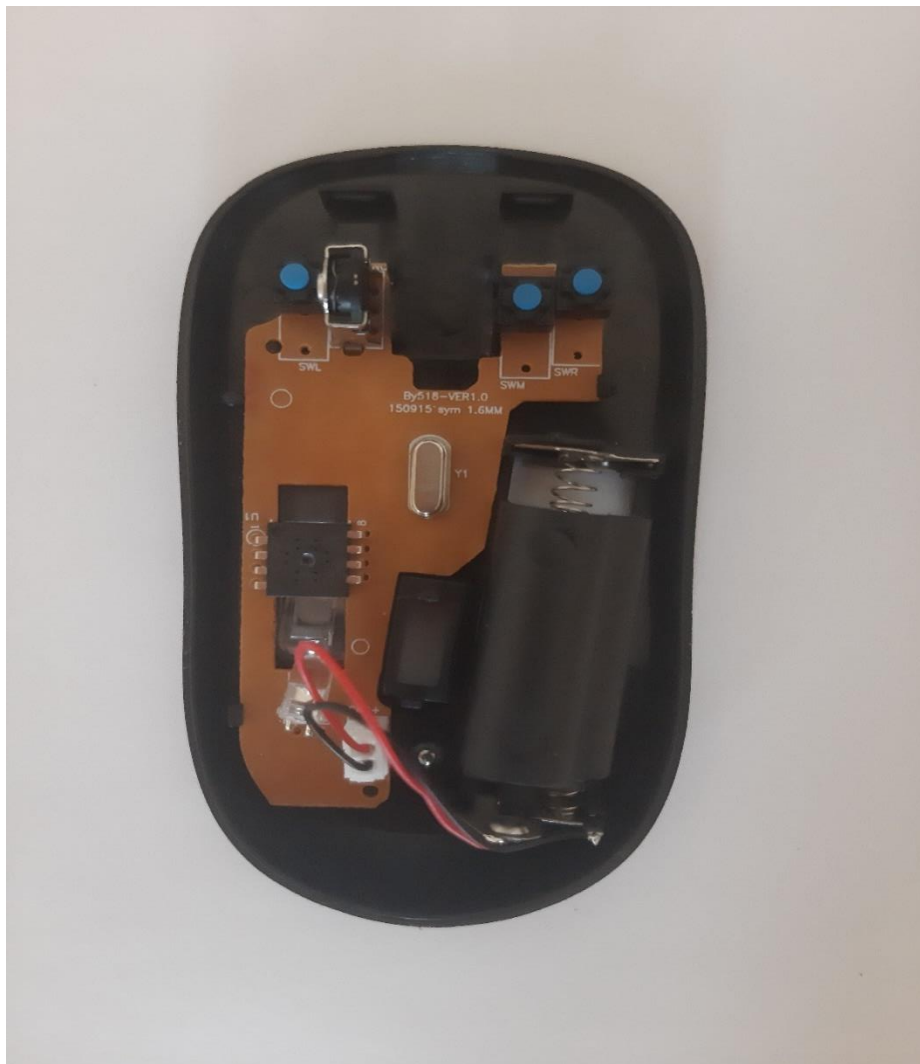
Figure 16 The inside of Hama mouse
