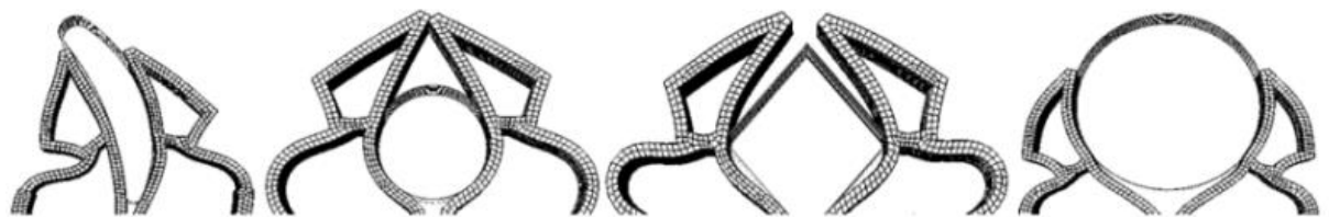
Figure 2.15 Verification of the gripper functions for different shapes of grasping objects [7]
