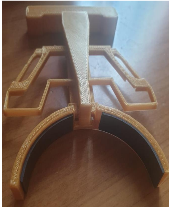
Figure 5.6 Gripper after magnet installation
