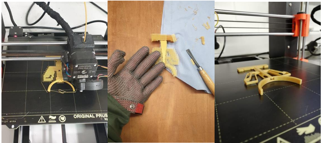
Figure 5.4 Process of 3D printing, support removing and final product
