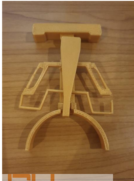
Figure 6.4 The CM broken when pressing too hard Vietnamese-German University
