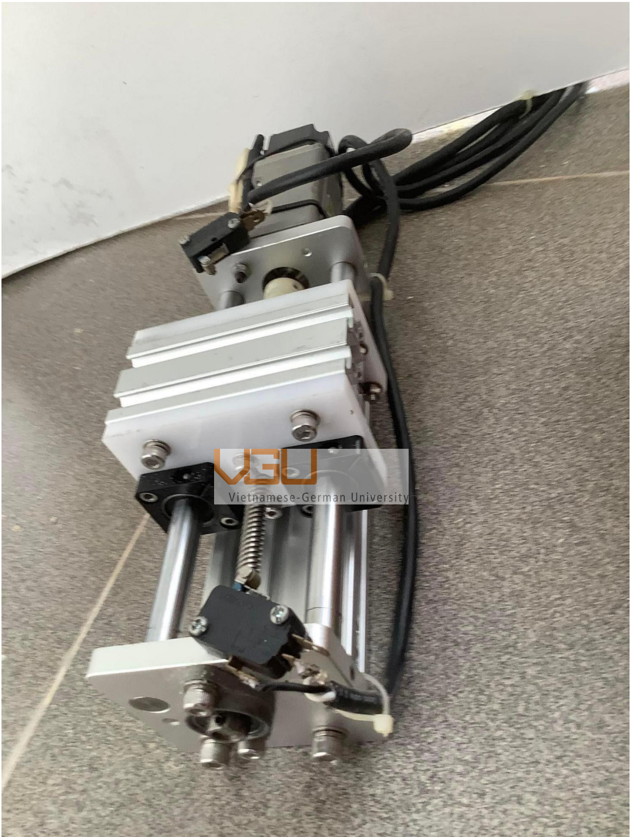
Figure 5.5: The Z axis with mount part for Y-Z connection.
