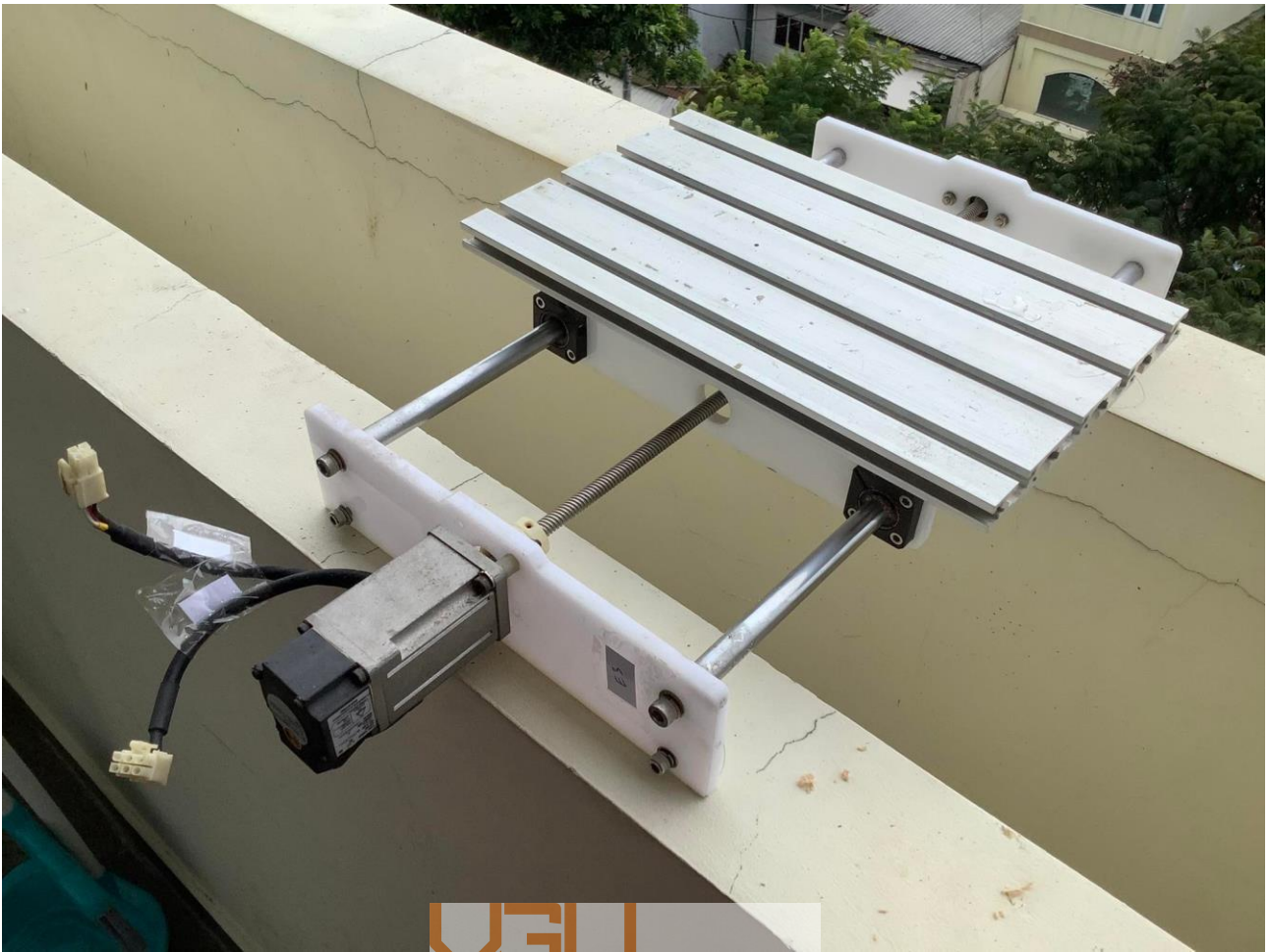
Vietnamese-German University Figure 5.2: The build of X axis linear movement.
