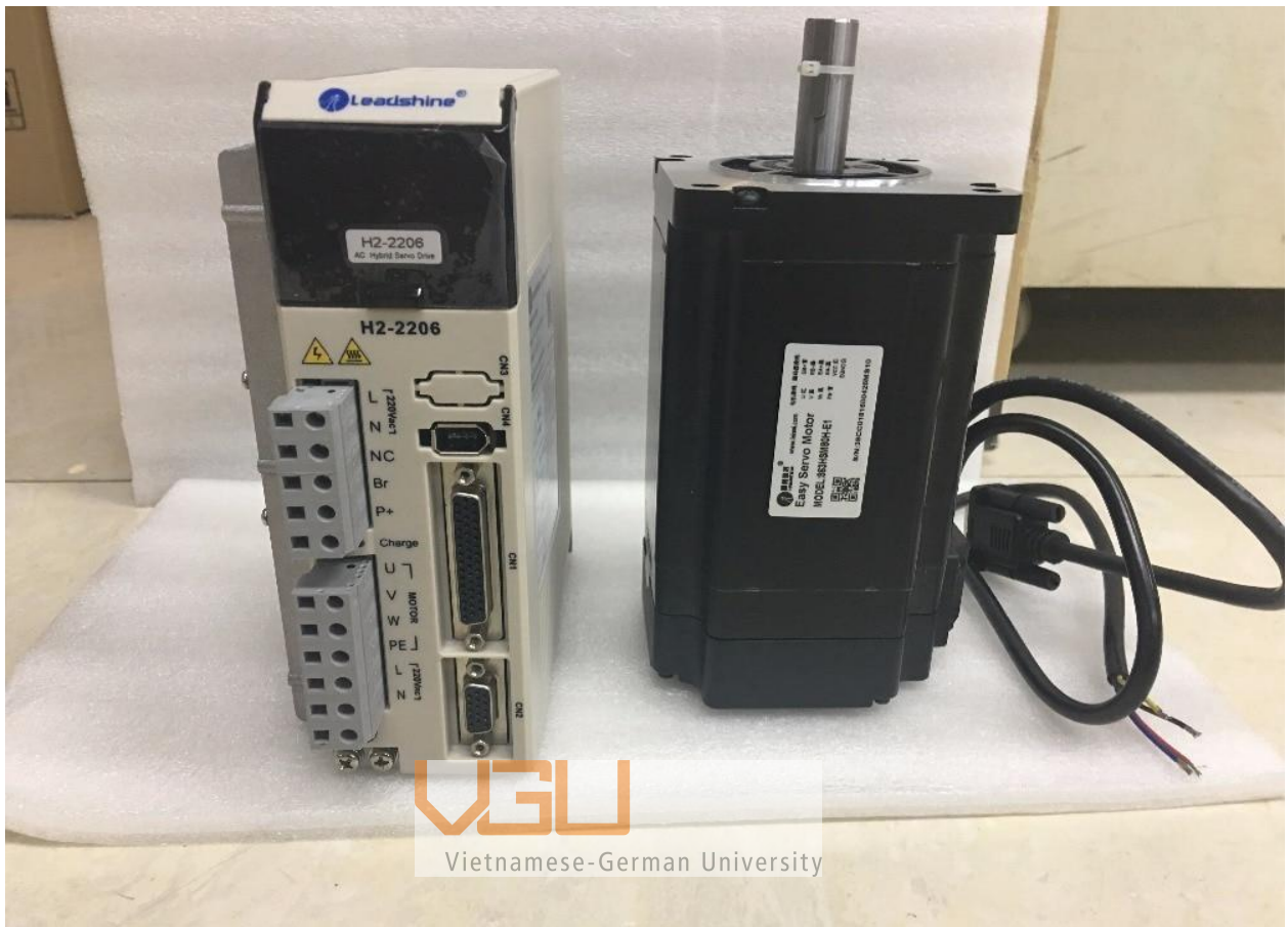
Figure 2.6: A pack of servo driver and its compatible AC drive.
