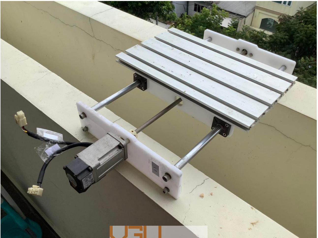
Vietnamese-German University Figure 3.3: The build of X axis linear movement.
