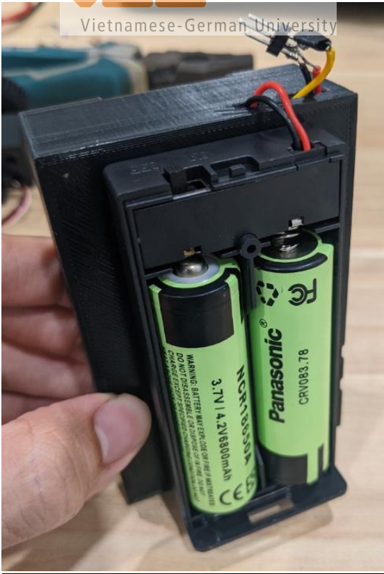
Figure 23: Battery case under electrical housing
